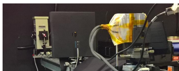
Figure 3. The angular response setup showing the Xe-Lamp in the back, a WG305 filter and a baffle in the middle and the JTSIM-DARA mounted on the goniometer.
